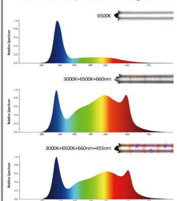
Adding an appropriate amount of infrared light to the SolarPro can enhance the accumulation of sugar in the plant body, making the fruit sweeter. Appropriate ultraviolet radiation can stimulate plant synthesis of plant hormones, carofenoids, anthocyanins, and other substances, improve photosynthesis efficiency and yield, and increase crop quality and yield. In addition, moderate amounts of ultraviolet radiation can also make plants produce more flowers and fruits.
